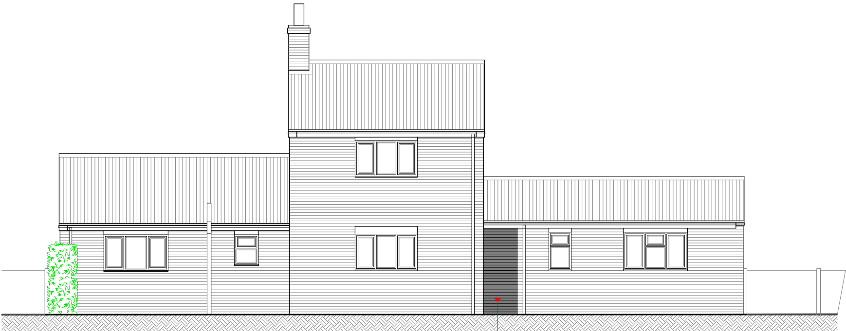
EXTENSION WALLS WITH FACING BRICKWORK TO MATCH EXISTING TO LINE THROUGH WITH CONSERVATORY WALLS WITH GLAZING REMOVED UPVC WINDOWS AND DOORS TO MATCH EXISTING
